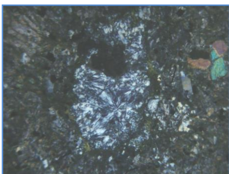
Figure (18) Microphotograph of Basalt showing spherulite texture (quartz) from Wilartha Taung (under XN, 40x).
